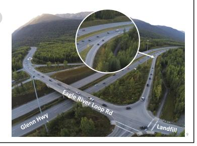
The existing southbound on-ramp merge operates near capacity as a tapered merge. This configuration has proven to be a challenge, especially during the morning peak traffic time. The situation is further compounded by the limited number of vehicles able to enter the Glenn Highway, as the single entrance lane and the tight left turn from Eagle River Loop Road create a significant bottleneck. As a result, the flow of traffic is hindered, leading to congestion and delays.
