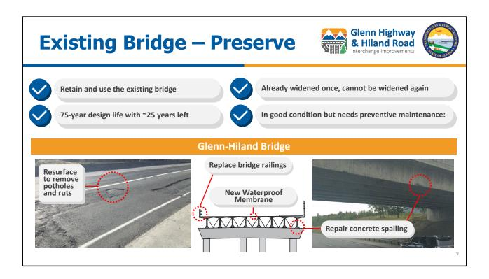
The existing bridge was constructed with a 75-year design life and has approximately 25 years remaining. This project will retain and use the existing bridge. As the existing bridge was already widened once, it cannot be widened again due to structural constraints. It is in good condition but needs preventive maintenance including:
